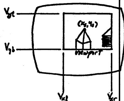
$$x_s = \frac{(x_w - w_{x1})}{(w_{xr} - w_{x1})} \cdot \underbrace{(v_{xr} - v_{x1})}_{\text{viewport width}} + v_{x1}$$
