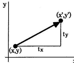
$$\begin{aligned} x' &= x + t_x \\ y' &= y + t_y \end{aligned}$$
