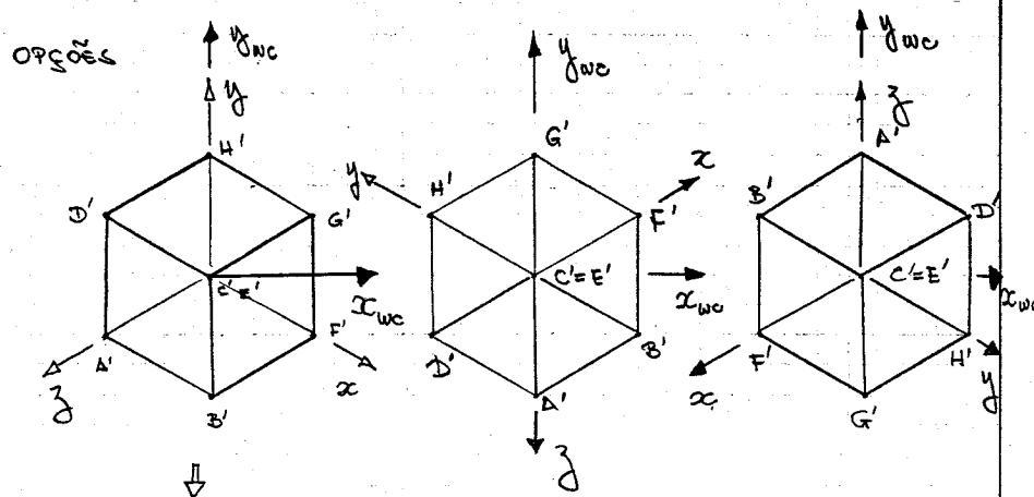
$$T \begin{pmatrix} 1 \\ 0 \\ 0 \end{pmatrix} = T(F) = F' = \begin{pmatrix} l \cos 30^\circ \\ -l \sin 30^\circ \\ 0 \end{pmatrix} = \begin{pmatrix} \frac{\sqrt{6}}{3} \frac{\sqrt{3}}{2} \\ -\frac{\sqrt{6}}{3} \frac{1}{2} \\ 0 \end{pmatrix} = \begin{pmatrix} 0.7071 \\ -0.4082 \\ 0 \end{pmatrix}$$
