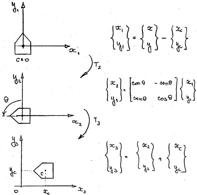
$$\begin{Bmatrix} x' \\ y' \\ \omega \end{Bmatrix} = \begin{bmatrix} \cos \theta & -\sin \theta \\ \sin \theta & \cos \theta \end{bmatrix} \left( \begin{Bmatrix} x \\ y \\ \omega \end{Bmatrix} - \begin{Bmatrix} x_c \\ y_c \\ \omega \end{Bmatrix} \right) + \begin{Bmatrix} x_c \\ y_c \\ \omega \end{Bmatrix}$$
