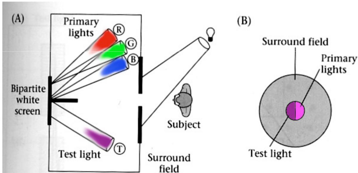
**4.10 THE COLOR-MATCHING EXPERIMENT.** The observer views a bipartite field and adjusts the intensities of the three primary lights to match the appearance of the test light. (A) A top view of the experimental apparatus. (B) The appearance of the stimuli to the observer. After Judd and Wyszecki, 1975.
