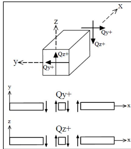
Figure 15: Positive internal shear force
