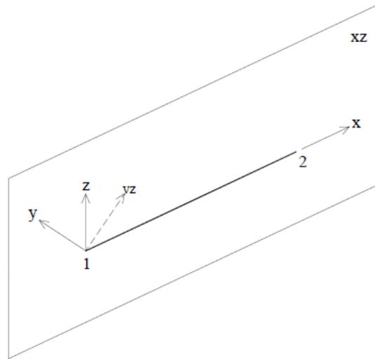
Figure 10: Local axes of elements in 3D models
