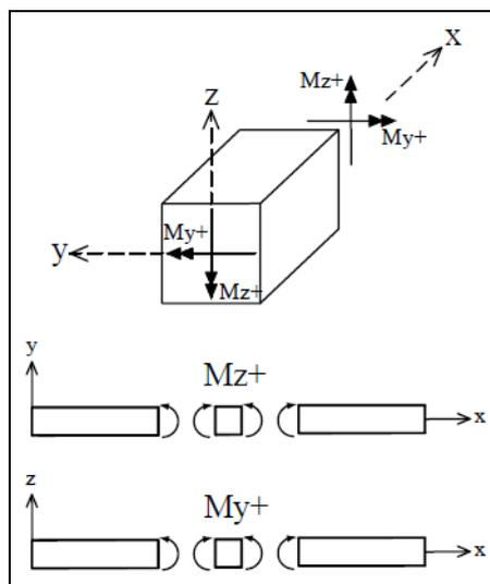
Figure 16: Positive internal bending moment
