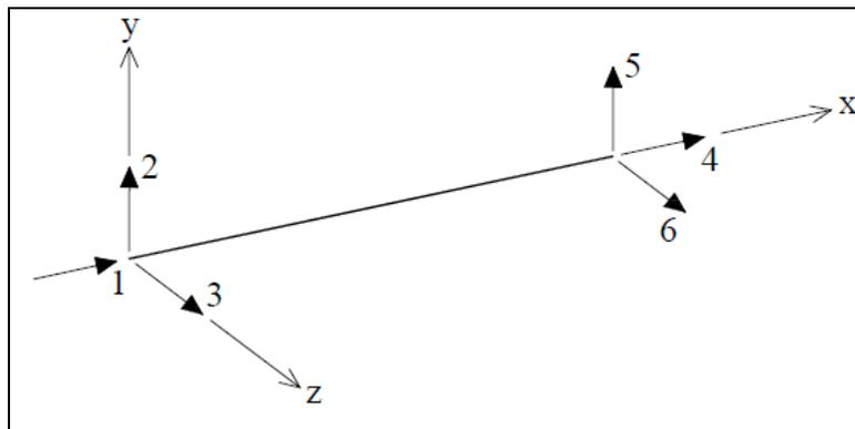
Figure 4: Degrees of freedom positive directions of a 3D truss element in local system
