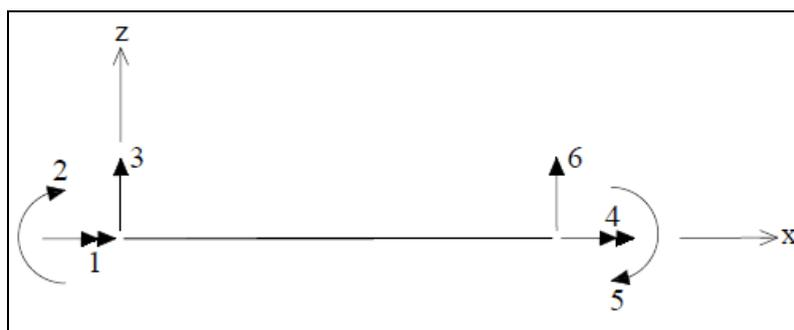
Figure 7: Degrees of freedom positive directions of a grillage element in local system
