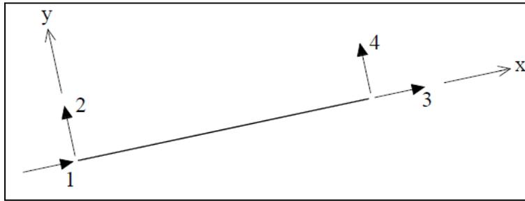
Figure 3: Degrees of freedom positive directions of a 2D truss element in local system
