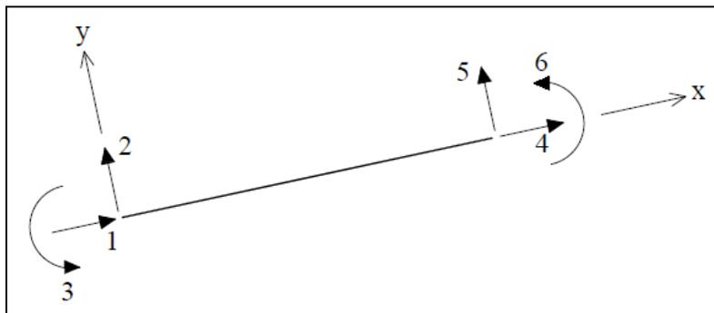
Figure 5: Degrees of freedom positive directions of a 2D frame element in local system
