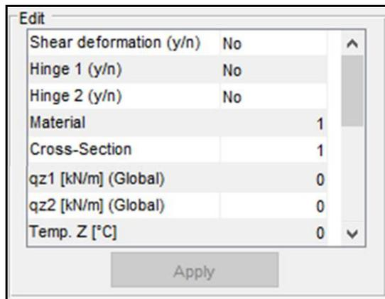
Figure 37: Editable informations of an element on a grillage model
