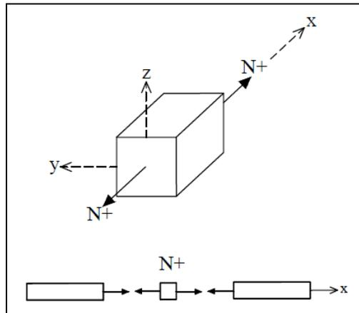
Figure 13: Positive internal axial force
