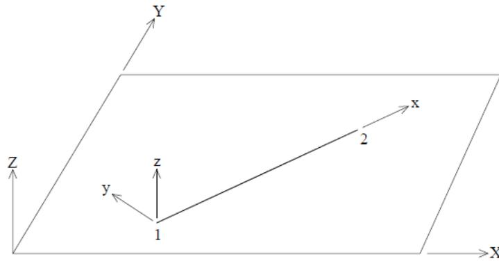
Figure 9: Local axes of elements in 2D models
