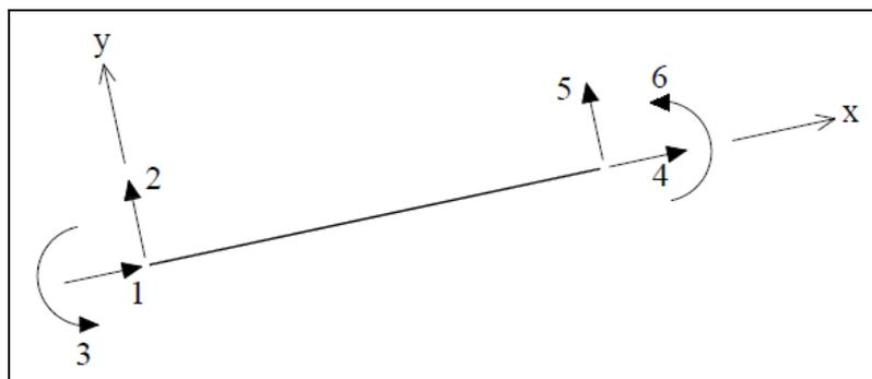
Figure 5: Degrees of freedom positive directions of a 2D frame element in local system
