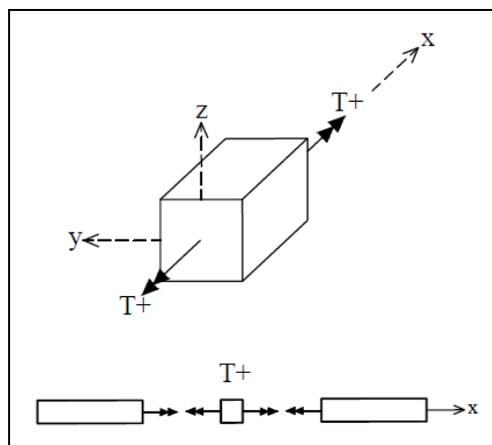
Figure 14: Positive internal torsion moment
