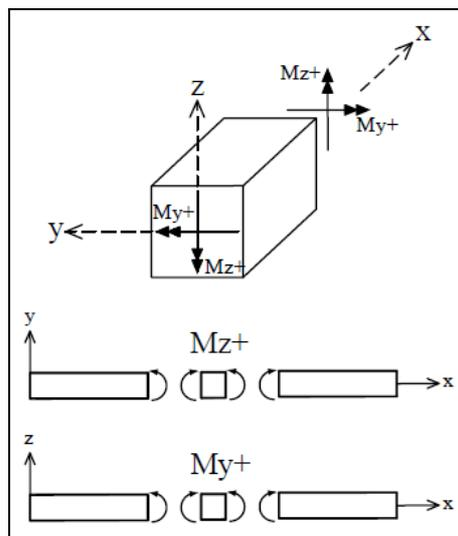
Figure 16: Positive internal bending moment
