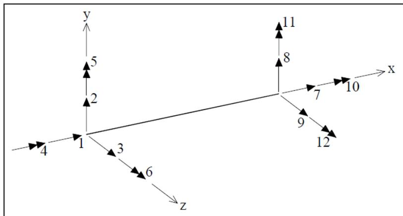
Figure 6: Degrees of freedom positive directions of a 3D frame element in local system
