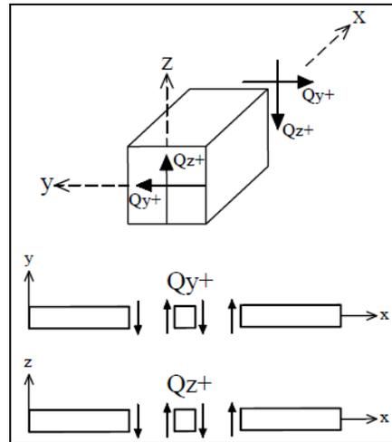
Figure 15: Positive internal shear force
