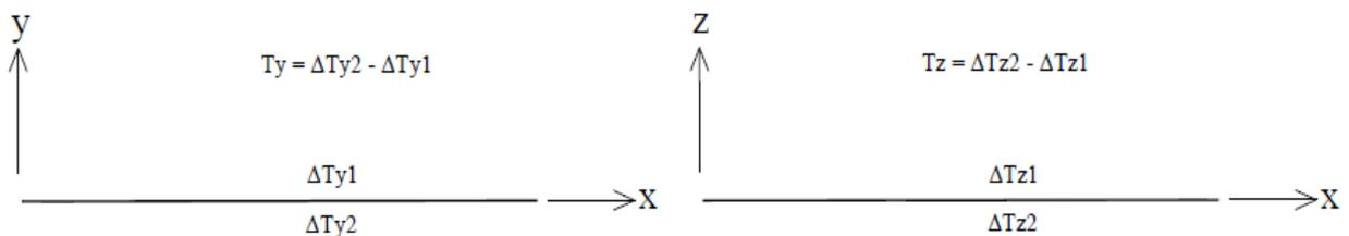
Figure 12: Temperature gradient convention
