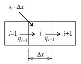
$$\left(-k\cdot A\cdot \frac{h_i-h_{i-1}}{\Delta x}\right) - \left(-k\cdot A\cdot \frac{h_{i+1}-h_i}{\Delta x}\right) = S_s\cdot \frac{\partial h_i}{\partial t}\cdot \Delta x\cdot A - s_i\cdot \Delta x$$
