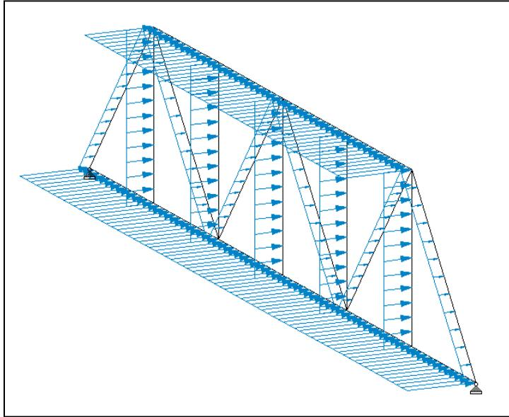
Figure 5.39 - Load diagram for wind on open structures
