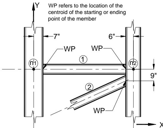
$f_1, f_2,$  and  $f_3$  correspond to the distance, measured in LOCALized or Global coordinate system, from the joint (START or END as specified) to the centroid of the starting or ending point of the members listed. MEMBER OFFSET command can be
