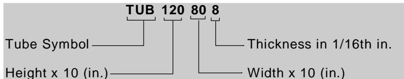
Tubes, like pipes, can be input by their dimensions (Height, Width and Thickness) as follows.
