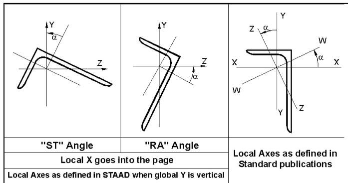
Figure 1.6a - Local axis system for various cross sections when global Y axis is vertical.
