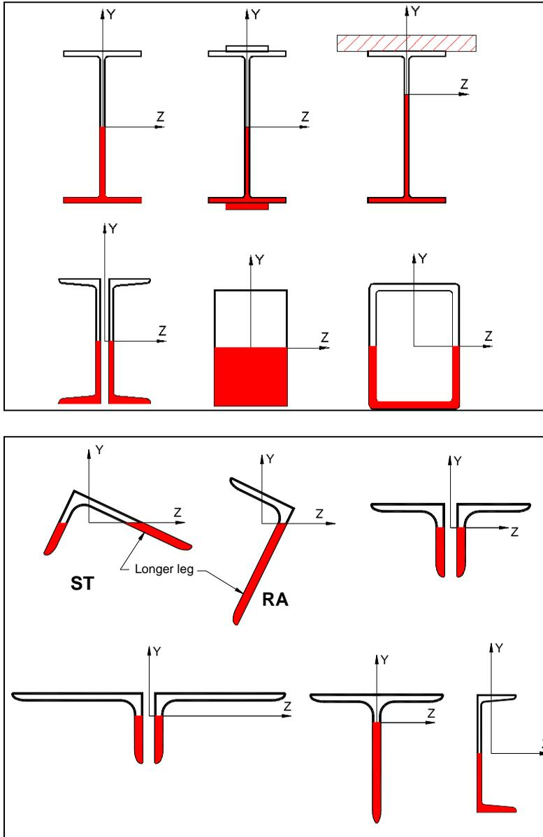
**Figure 1.41 - Stress Zones due to bending about Z axis (MZ)**
