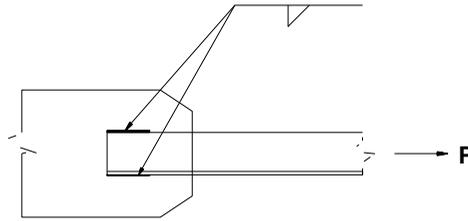
Figure 2.4 - Weld design for SELECT WELD TRUSS.
