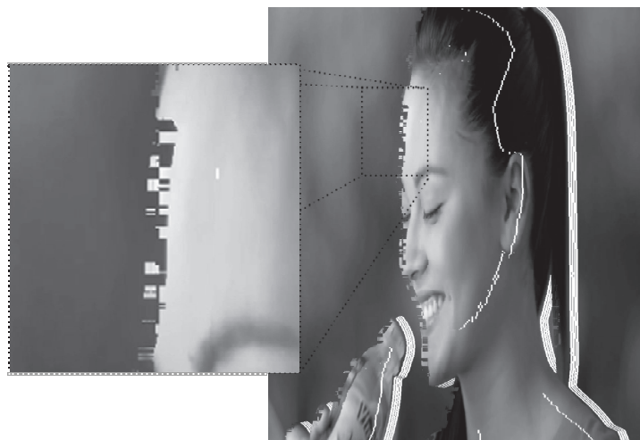
Fig. 3. Example of warping multiple pixels to the same target position without a thread-safe access to the depth buffer (the frame is shown without hole filling) 1
