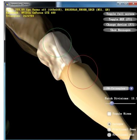
Figure 10: PN-Triangles with linearly interpolated normals
