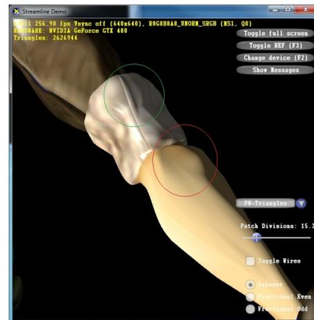
Figure 11: PN-Triangles with quadratic normals interpolation
