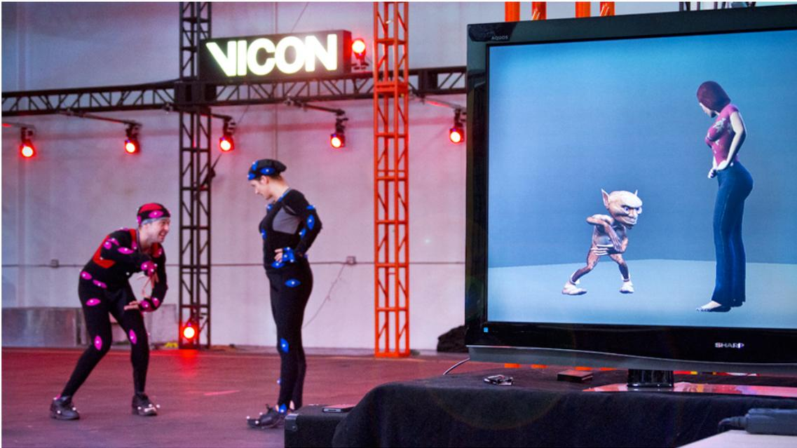
Figure 2.2: Vicon Motion Capture System.
