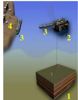
Figure 1: (1) reservoir; (2) offshore platform; (3) transportation ships; (4) oil pipelines.
