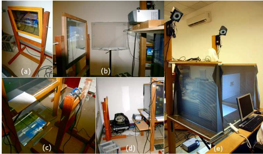
Fig. 13 (a) Mirrors in MiniCave. Pair Projector/Mirror on screens: (b) frontal, (c) under the table and (d) sides. (e) Overview of the HybridDesk structure during its development
