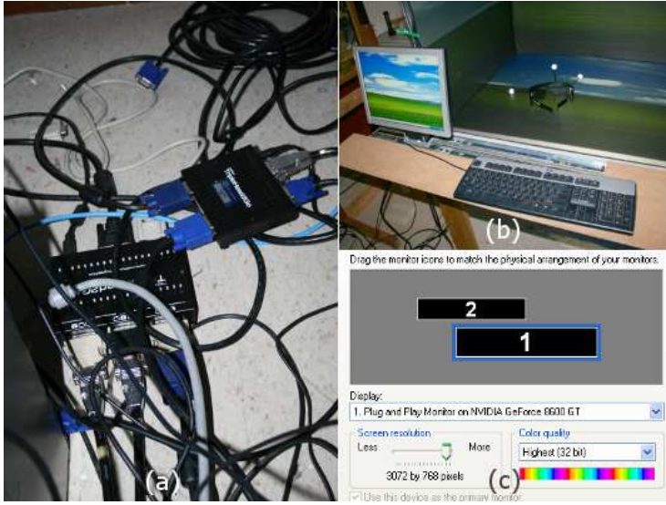
Fig. 8 (a) Two Matrox TripleHead2Go splitters to extend (b) the desktop through all the screens (c) using only one graphics board with two video outputs.
