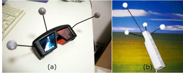
Fig. 10 (a) Anaglyphic Stereo Glasses and (b) Wiimote used as a Wand.
