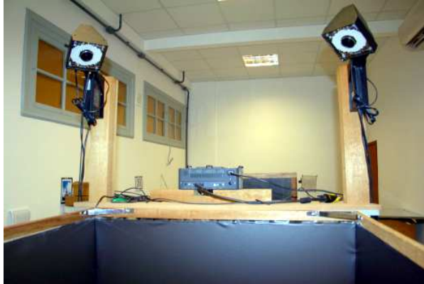
Fig. 9 Optical Tracker composed by two infrared cameras.
