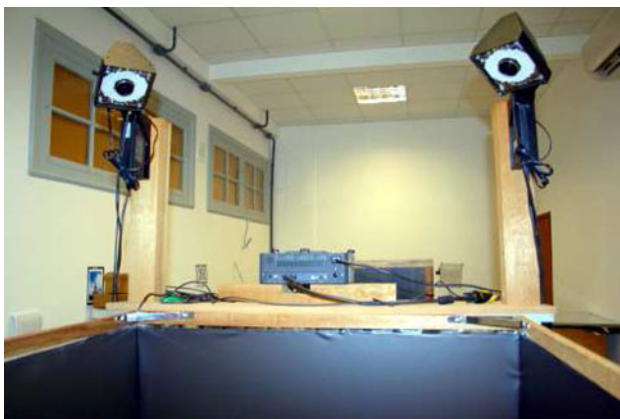
Fig. 9 Optical tracker composed by two infrared cameras
