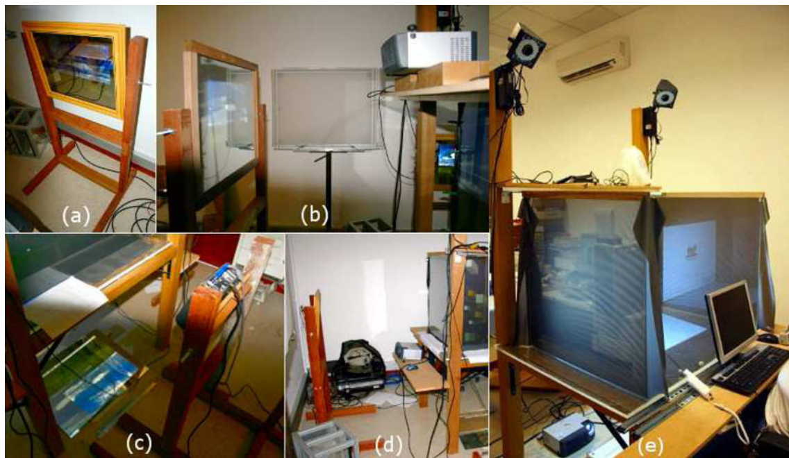
Fig. 13 a Mirrors in the MiniCave. Projector/mirror pairs for the screens: b front, c under the table, and d sides. e Overview of the HybridDesk structure during its development
